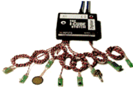
Figure 2: The I-Cube System Digitizer and a few sensors. Courtesy Infusion Systems Ltd. [60].
